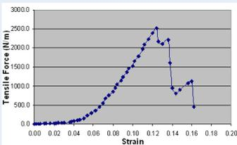
Figure 6: Tensile test with very flexible end-fixing
