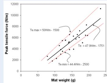
Figure 8: Correlation of initial tensile strength and weight
