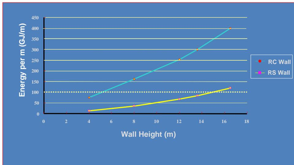
**Figure 10.** Comparison of the embodied energy of reinforced soil v reinforced concrete walls (After Geoguide 6, 2002)
