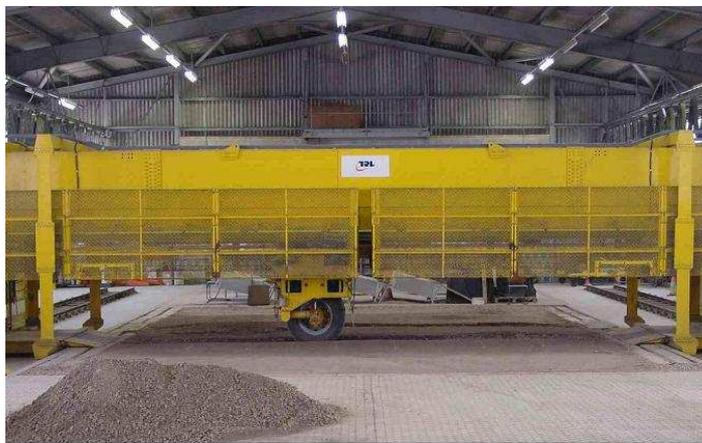
**Figure 2.** Accelerated Pavement Testing at TRL
