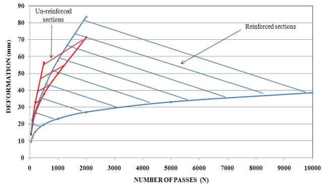
**Figure 5.** Range of deformations in the wheel path
