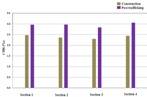
**Figure 4.** Change in stiffness of the subgrade
