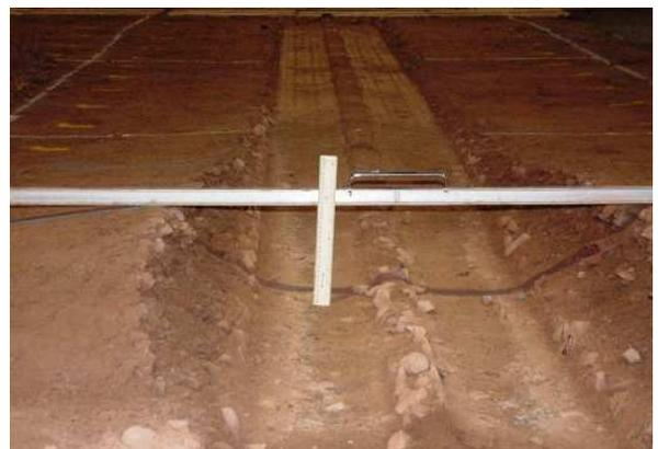
**Figure 7.** Measurement of rut depth
