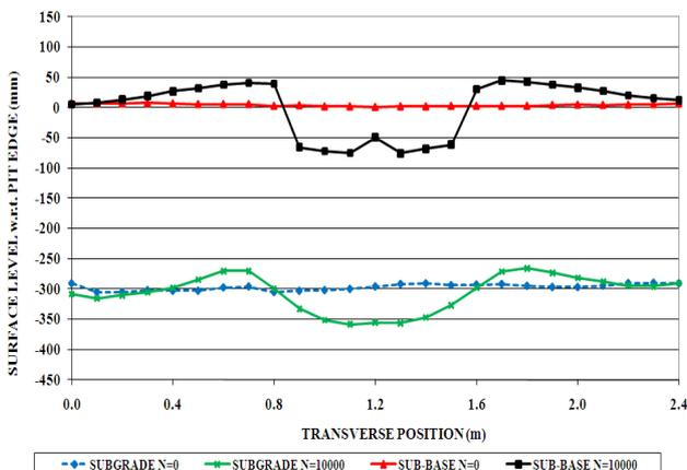
**Figure 6.** Deformation of the sub-base and subgrade
